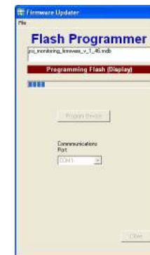
On PC Flash Programmer uploading firmware into 5200A
