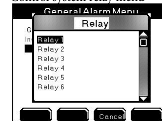
Control system relay menu
