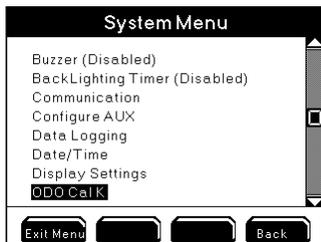
Cap calibration codes are not stored in the 5500D instrument but rather are stored in the ODO sensor. Upon selecting DO-1, DO-2, DO3 or DO-4 at the ODO Cal K menu, communication initiates between the instrument and the sensor. An ODO sensor has six cap calibration codes. They are known as K1, K2, K3, K4, K5 and KC.
