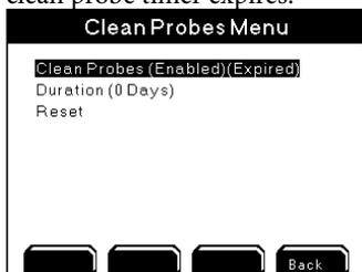
Reset Clean Probe timer at the
