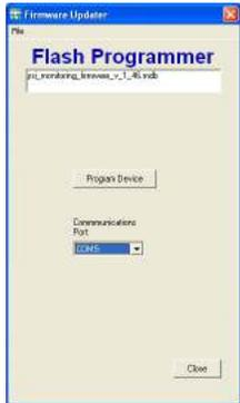
6. AquaManager Program Folder includes the latest version of instrument firmware. The latest firmware is stored as an .mdb file in the PC Program Files>AquaManager>Firmware. At AquaManager, Firmware Updater>File>Load Firmware Database. Locate and load this file into the Firmware Updater.
