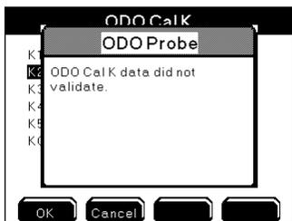
6. If no validation error message is displayed, the ODO calibration codes were entered correctly. **Exit Menu** to save and return to run screen.
