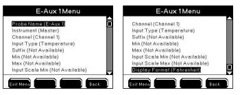
Configure E-Aux temperature Configure E-Aux system menu:
