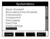
Cap calibration codes are not stored in the 5500D instrument but rather are stored in the ODO sensor. Upon selecting DO-1, DO-2, DO3 or DO-4 at the ODO Cal K menu, communication initiates between the instrument and the sensor. An ODO sensor has six cap calibration codes. They are known as K1, K2, K3, K4, K5 and KC.
