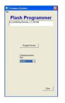
6. AquaManager Program Folder includes the latest version of instrument firmware. The lastest firmware is stored as an .mdb file in the PC Program Files>AquaManager>Firmware. At AquaManager, Firmware Updater>File>Load Firmware Database. Locate and load this file into the Firmware Updater.
