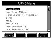
5500 Configure Aux 5 menu (Temp Source menu will be available when Temperature Input Type configured
