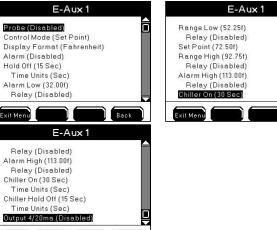
5400 5400 only - Aux configured temperature systems can be configured as the temperature compensation source for any of the four DO channels. Aux configured temperature systems can also be configured as independent temperature systems at any location in the system stream.
