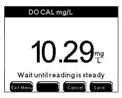
After one minute, verify that the DO value shows no significant change for approximately 30 seconds. Then, press Next to complete the calibration OR press Cancel to escape calibration and return to calibration menu without saving.
