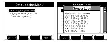
In the above sensor log screen shot Aux 3 is assigned as temperature for DO 1. DO 4 and Aux 1, 2, 4, 5, & 6 are disabled.
