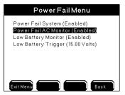
Disabling the *Power Fail System* will disable AC power events and disable the General Alarm in the event of low battery for DC power. *Disable Power Fail AC Monitor* when powering 5X00 by a DC power source.
