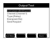
3. dt Instrument menu. Device Address menu opens. Scroll and select networked instrument whose relay or channel is to be tested.
