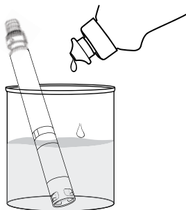
Figure 73 Cleaning the pH and pH/ORP sensor with dish soap
