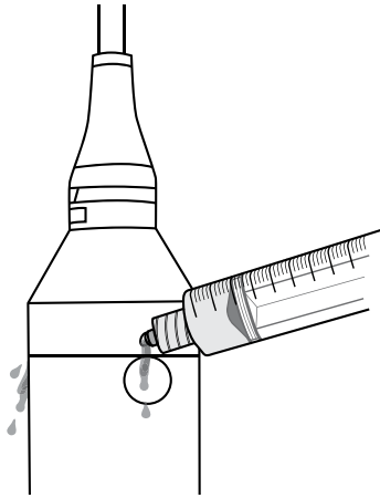
Figure 65 Depth sensor flush
