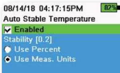
Figure 33 Auto Stable stability threshold
